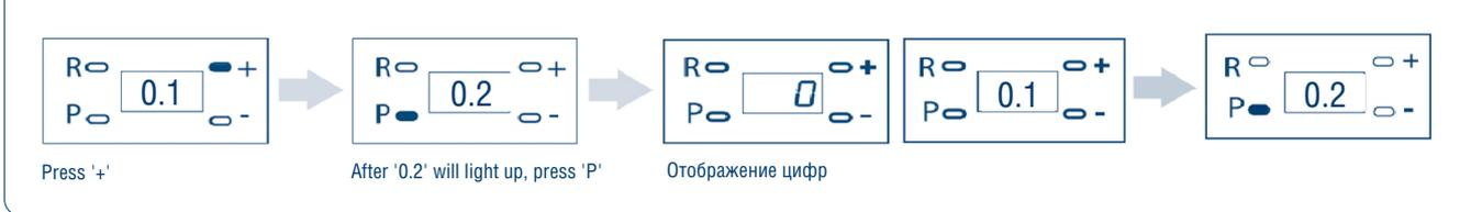
Once you access menu option '0.2', the display will show four numbers, one after the other. This value indicates the total number of open/close cycles the operator has performed since it was manufactured.
