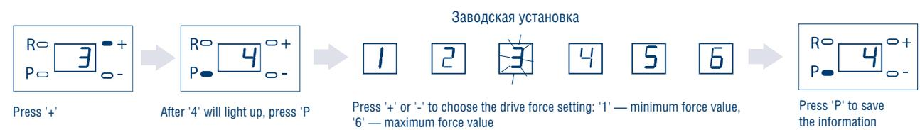
By default, the drive is set to force level three; users generally do not need to adjust these settings.
